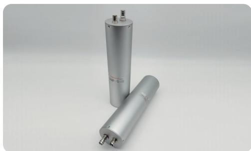
EPS-D50H50VD01 scintillator detector is composed of 2-inch plastic scintillator, photomultiplier tube, and voltage divider. Due to its high sensitivity, flexible matching, simple use, and stable performance, it is widely used in radiation protection, site monitoring, nuclear medicine, nuclear power plants and other fields.
