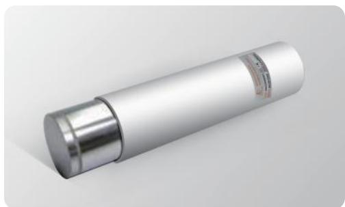
The ENAI-D50H50DHP01 scintillator detector is a highly integrated detector composed of a 2-inch Nal scintillator, photomultiplier tube, voltage divider, high-voltage module, and preamplifier. It can be used for gamma ray energy spectrum measurement, directly output negative polarity signal. Due to its high detection efficiency, good energy resolution, and stable performance, it is widely used in energy spectrum measurement analysis, densitometry, coal ash analysis and other fields.
