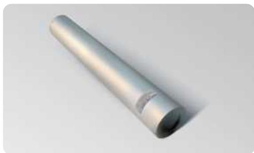
The ENAI-D25H25DHP01 scintillator detector is a highly integrated scintillator detector composed of a 1-inch Nal scintillator, photomultiplier tube, voltage divider, high-voltage module, preamplifier. It can be used for gamma ray energy spectrum measurement, directly output negative polarity signal. Due to its small size, good resolution, simple use, and high reliability, it is widely used in fields such as radiation safety detection and precision measurement analysis.
