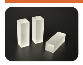
Cerium doped silicate yttrium, YSO(Ce), belongs to monoclinic rare earth ortho-silicate crystal, it is similar with the LYSO(Ce) crystal, while generally used as a semiconductor and in photo optic applications. YSO(Ce) crystal shares the same emission peak 420 nm with LYSO(Ce), but it is less efficient in terms of light output, which is around 28,000 Photons/MeV, the decay time of YSO(Ce) 50-70 ns is slower than LYSO(Ce)'s 40 ns.
